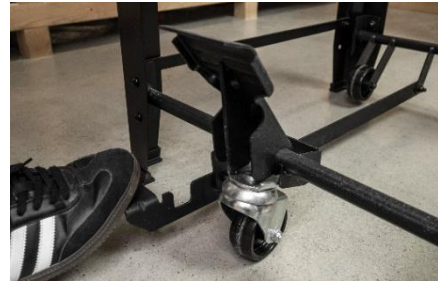
Fig. 11. Pedal up – the stand rests on its legs and the wheels are raised.
